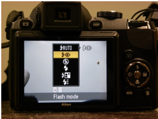
Figure 6. This camera has a mode designed to reduce the “red eye” effect when using a flash.
